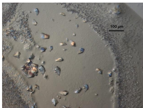
Figure 10. Crystallization trial of ShuA at 5 mg.mL -1 in 50 mM Tris pH 7.5, 150 mM NaCl, 0.5 mM DDM using the vapor-diffusion technique (reservoir solution: 35% PEG 300, 100 mM NaCl, 100 mM Na-Citrate pH 5 ; hanging droplet: 1μL ShuA-DDM)
